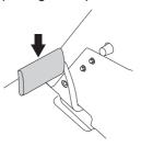
2 Carefully press down one of the pedals until the required speed is obtained. Pedal (1) is used to drive forwards, and pedal (2) to drive backwards.
